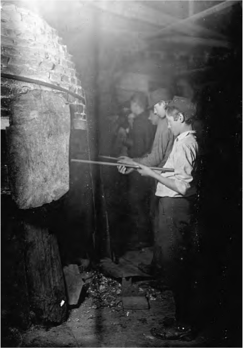
Boys at the "glory hole," where glass pieces were reheated before going to a finisher, 1908. (Library of Congress)
